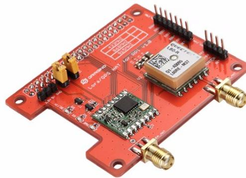
Figura 13 – Dragino LoRa/GPS *Hat* para Raspberry Pi.
