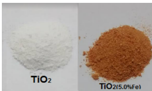
Figure 26 – a) Experimental Set-up and b) TiO_2 and Fe -doped TiO_2 in powder form.
