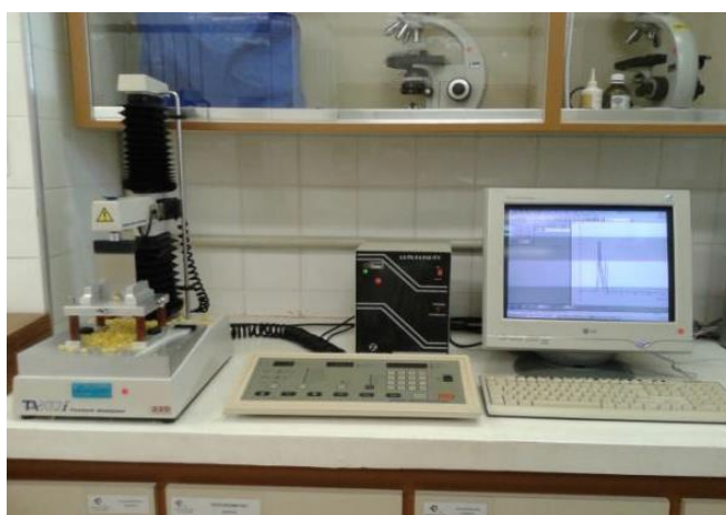
Figura 11: Textura Analyser (Extralab Brasil) equipado com o software Texture Expert®, Santos (2014).
