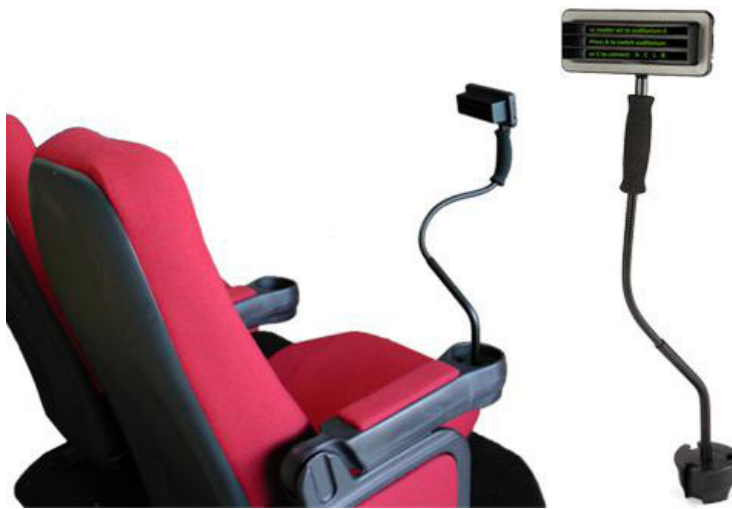
Figure 7 – CaptiView Closed Caption Viewing System for the DHH movie audiences (6).
