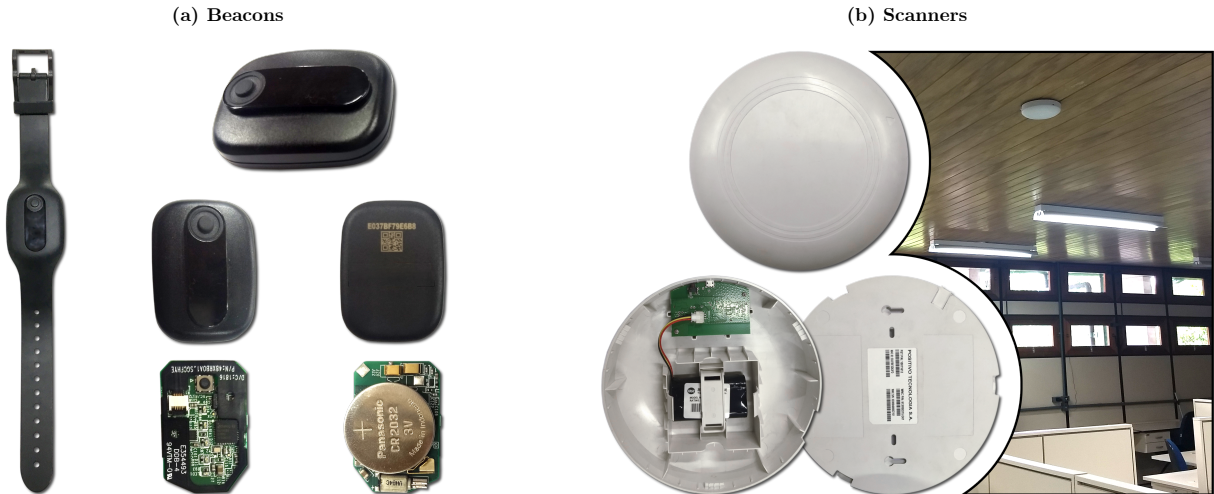
Figure 6: SmartCampus Hardware: (a) beacons with Bluetooth communication; one beacon is inside a bracelet, as used by the users; the other beacons are outside the bracelet (front and back), and opened to show hardware (front and back); and (b) scanners with Bluetooth and 900Mhz long-range communication (front, opened, back, and installed on the ceiling). The gateway has a similar hardware footprint as of the scanners, and the server is not shown.
